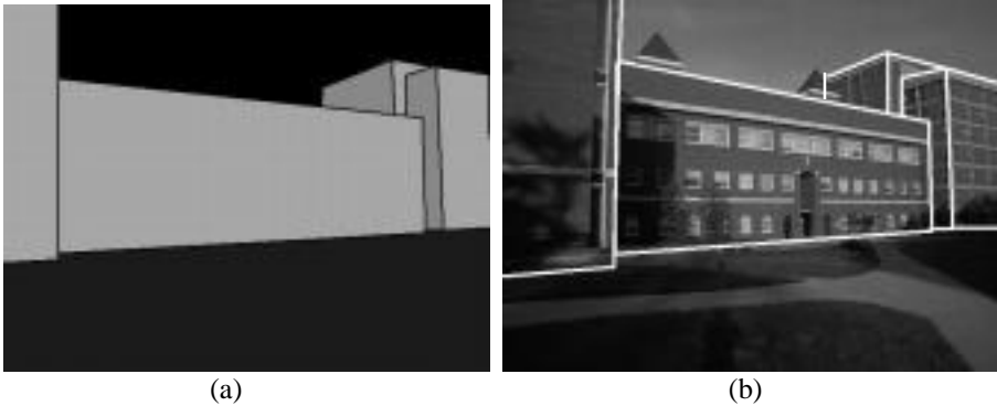
Fig. 17. (a) Baseline model as seen from recovered viewing position. (b) Baseline model edges backprojected into ground-level view using the recovered viewing parameters for subjective evaluation of accuracy.
