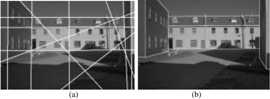
Fig. 13. (a) Salient line pencils. (b) Model lines, backprojected into ground-level view using the recovered viewing parameters.
