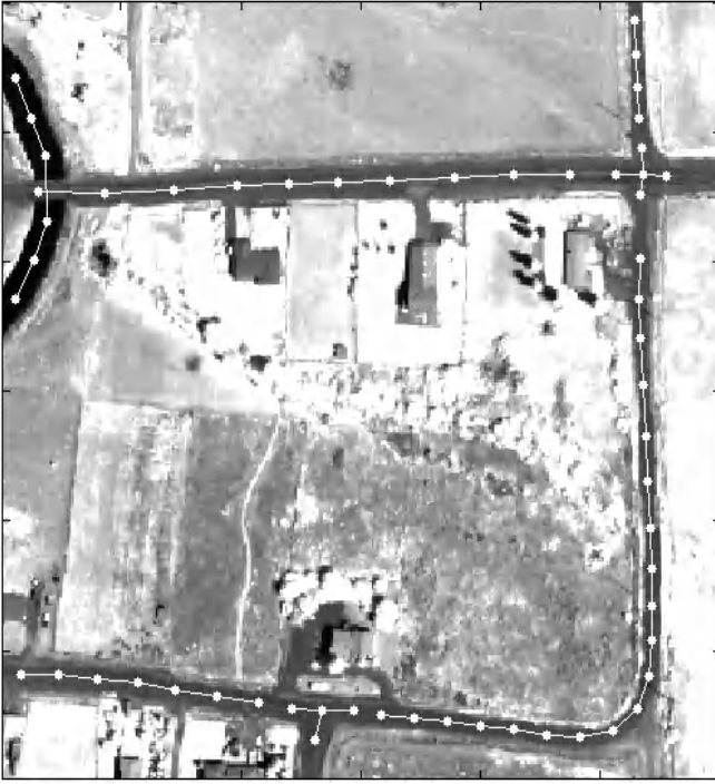
Fig. 8. SOM nodes for extracted linear feature components in the image
