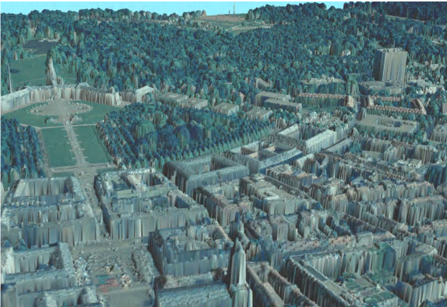
Fig. 3. 3D view of laser altimeter data textured by an aerial image
