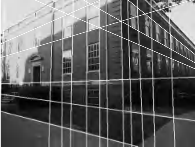
Fig. 8. Set of salient line pencils used to align terrestrial view with the initial model.
