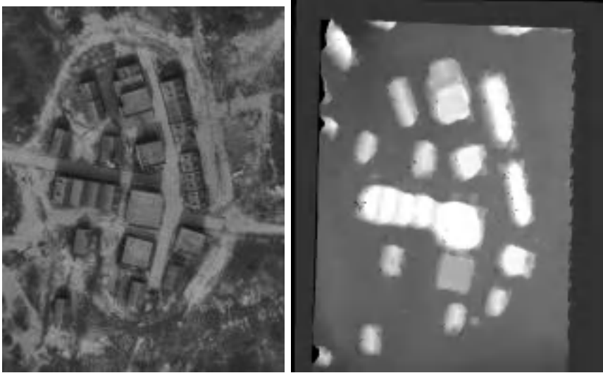
Fig. 2. Downlooking view of built-up area (left) and corresponding digital elevation map (right) Initial model acquisition requires calibrated aerial images and a digital elevation map (DEM) 1 .
