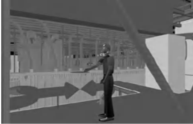
Figure 1: Interactive collision detection and tolerance verification between a user and the pipes in the power plant using IMPACT.
